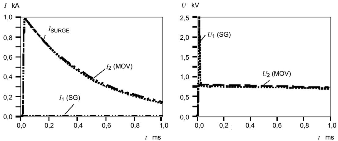
Figure C.6a – Current and voltage of spark gap and MOV from a 10/350  $\mu$ s surge (SPD 1 not ignited)
