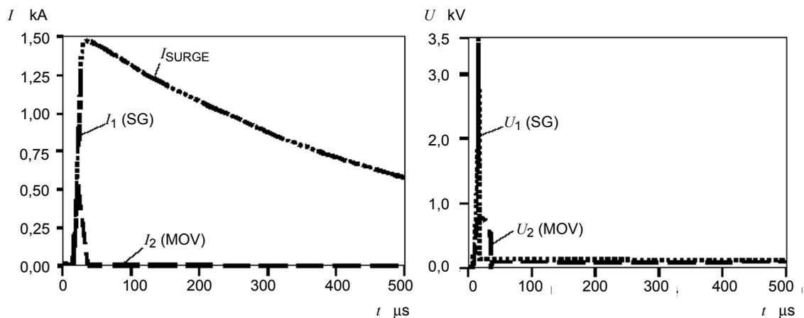
Figure C.6b – Current and voltage of spark gap and MOV from a 10/350  $\mu$ s surge (SPD 1 ignited)
