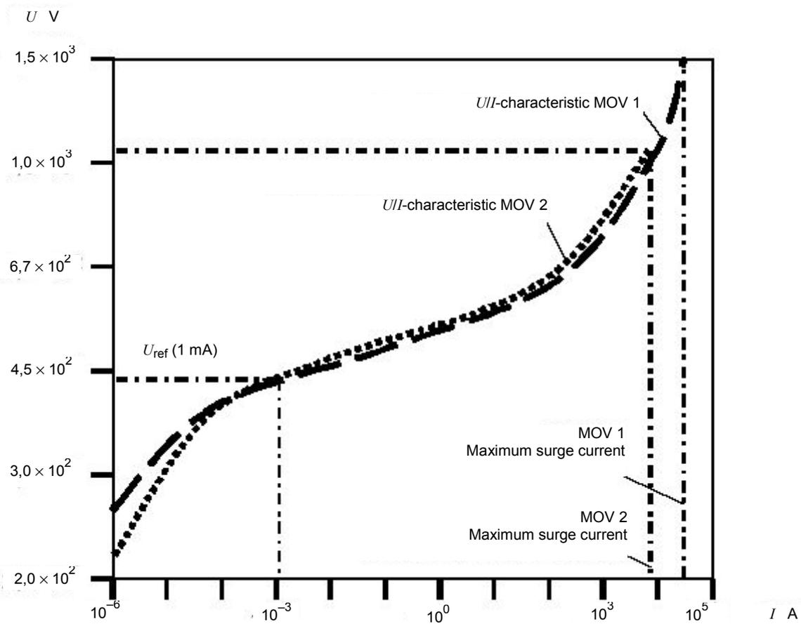
NOTE As can be seen in this example, the knowledge of the MOV's reference voltage  $U_{ref}$  only, is not sufficient for coordination purposes.
