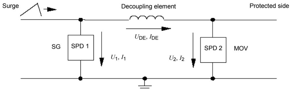
Figure C.5a – Circuit with spark gap and MOV
