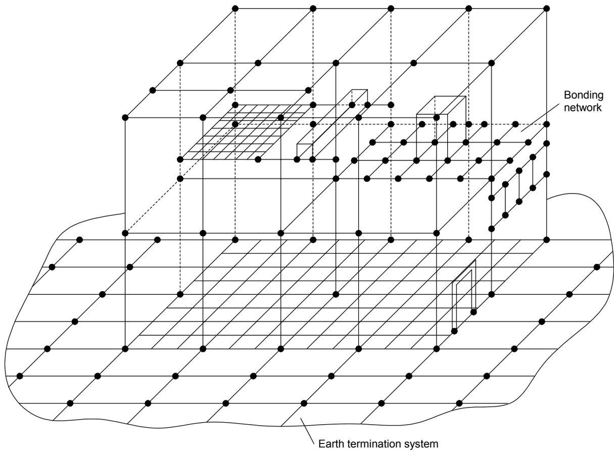
NOTE All drawn connections are either bonded structure metal elements or bonding connections. Some of them may also serve to intercept, conduct and disperse the lightning current into the earth.
