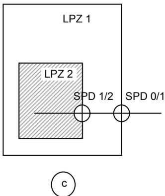
NOTE Figure 4c shows an LPZ 2 supplied by an electrical or signal line. This line needs two coordinated SPDs: one at the boundary of LPZ 1, the other at the boundary of LPZ 2.
