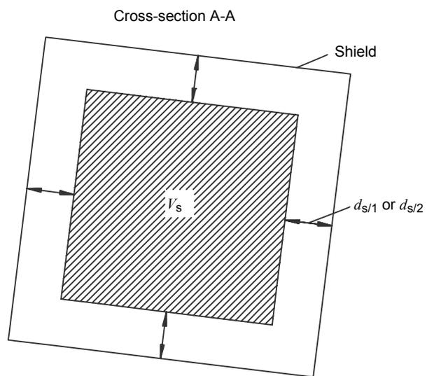
NOTE The volume  $V_s$  keeps a safety distance  $d_{s/1}$  or  $d_{s/2}$  from the shield of LPZ n.
