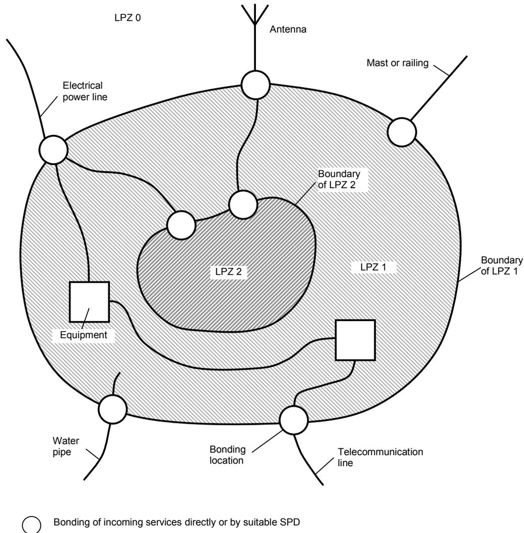
NOTE This figure shows an example for dividing a structure into inner LPZs. All metal services entering the structure are bonded via bonding bars at the boundary of LPZ 1. In addition, the conductive services entering LPZ 2 (e.g. computer room) are bonded via bonding bars at the boundary of LPZ 2.
