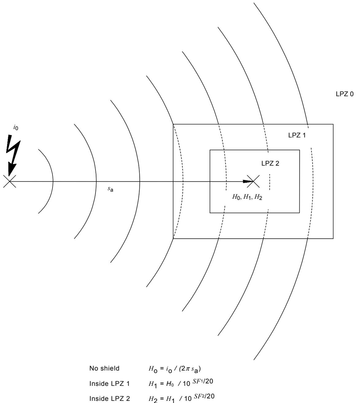
**Figure A.8 – Evaluation of the magnetic field values in case of a nearby lightning strike**
