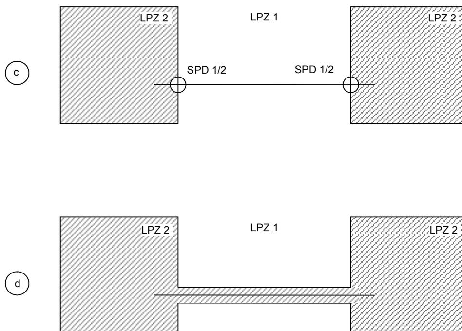
NOTE Figure 3c shows two LPZ 2 connected by electrical or signal lines. Because the lines are exposed to the threat level of LPZ 1, SPD at the entry into each LPZ 2 are required.
