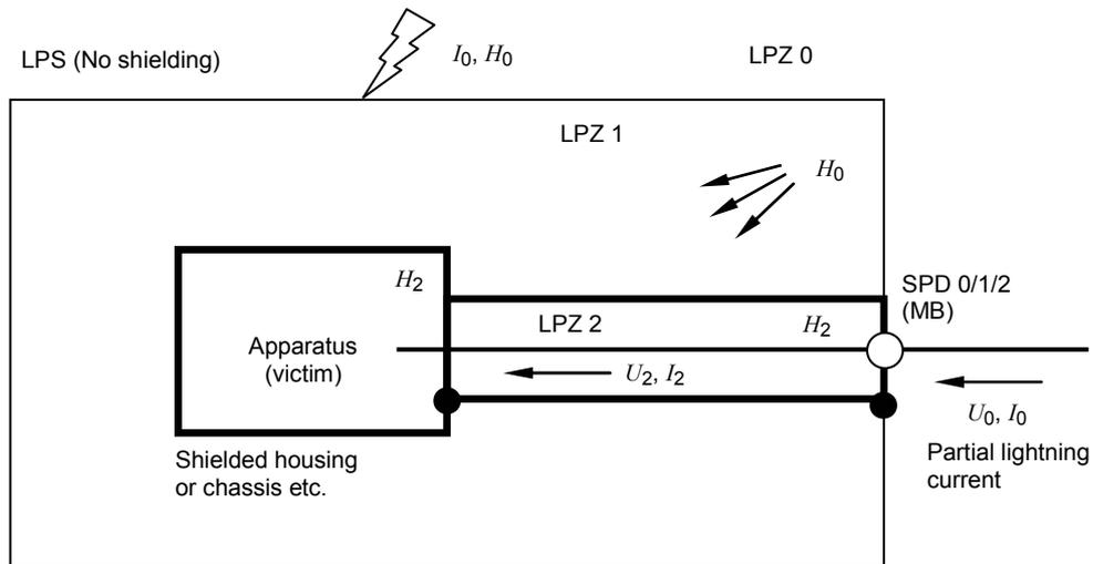
Figure 2c – LPMS using internal line shielding and SPD protection at entry of LPZ 1 – Apparatus protected against conducted surges ( $U_2 < U_0$  and  $I_2 < I_0$ ) and against radiated magnetic fields ( $H_2 < H_0$ )
