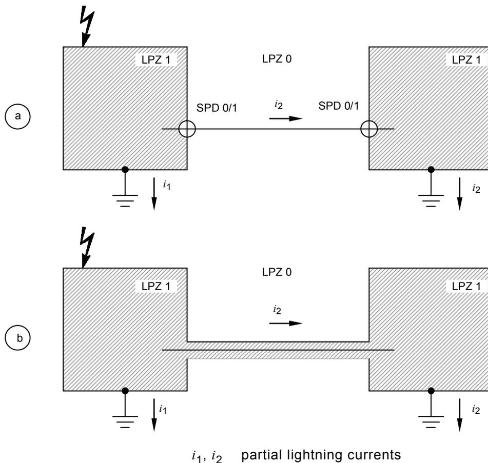
NOTE Figure 3a shows two LPZ 1 connected by electrical or signal lines. Special care should be taken if both LPZ 1 represent separate structures with separate earthing systems, spaced tens or hundreds of metres from each other. In this case, a large part of the lightning current can flow along the connecting lines, which are not protected.
