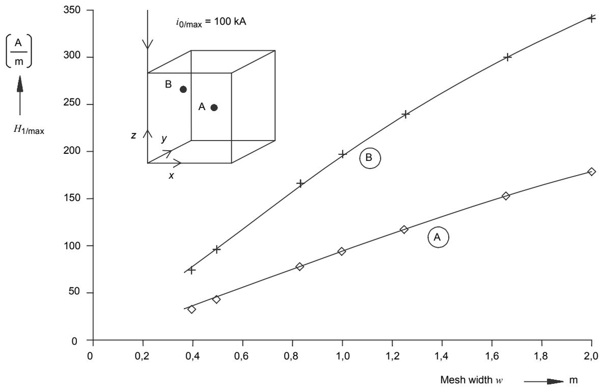
Figure A.12 – Magnetic field strength  $H_{1/\max}$  inside a grid-like shield Type 1
