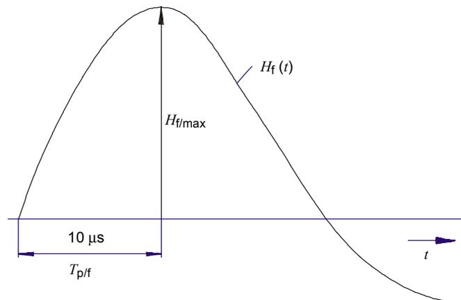
**Figure A.2a – Simulation of the rise of the field of the first stroke (10/350 μs) by a single impulse 8/20μs (damped 25 kHz oscillation)**
