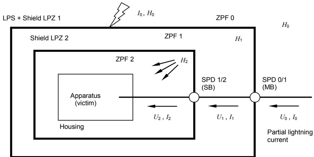
Figure 2a – LPMS using spatial shields and “coordinated SPD protection”– Apparatus well protected against conducted surges ( $U_2 \ll U_0$  and  $I_2 \ll I_0$ ) and against radiated magnetic fields ( $H_2 \ll H_0$ )
