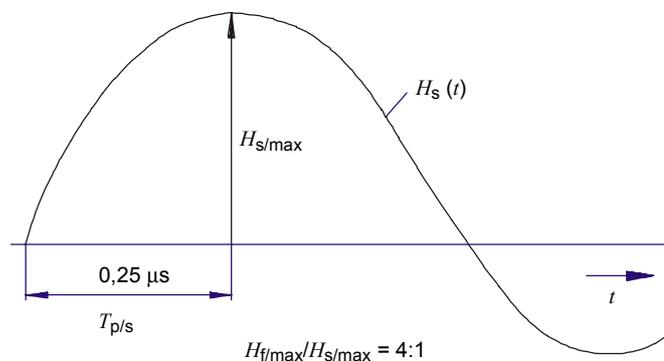
**Figure A.2b – Simulation of the rise of the field of the subsequent stroke (0,25/100 μs) by damped 1 MHz oscillations (multiple impulses 0,2/0,5μs)**
