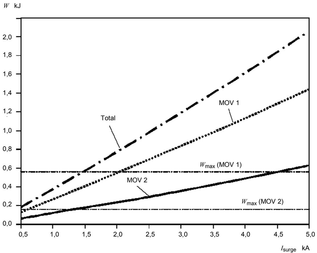
Figure C.3b – Principles of energy coordination between MOV 1 and MOV 2
