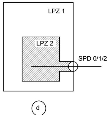
NOTE Figure 4d shows that the line can enter immediately into LPZ 2 and only one SPD is required, if LPZ 2 is extended into LPZ 1 using shielded cables or shielded cable ducts. However this SPD will reduce the threat immediately to the level of LPZ 2.
