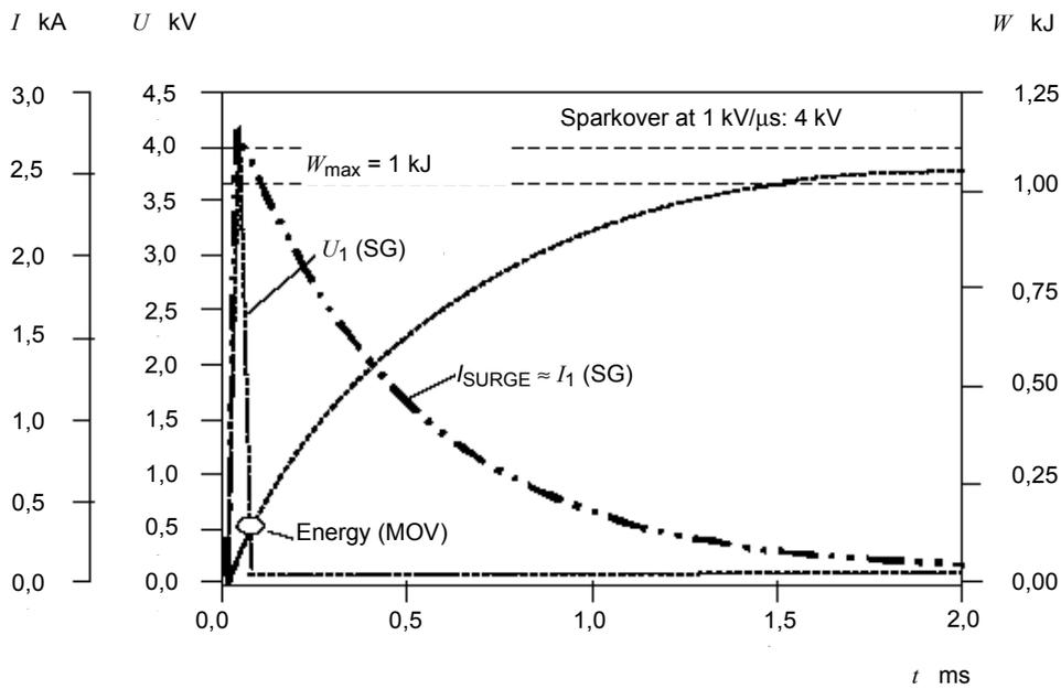
Figure C.8c – Current/voltage/energy characteristics for  $L_{DE} = 10 \mu H$  – Energy coordination for a 10/350  $\mu s$  surge achieved (spark gap ignited)
