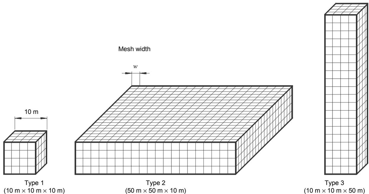
**Figure A.10 – Types of grid-like large volume shields**
