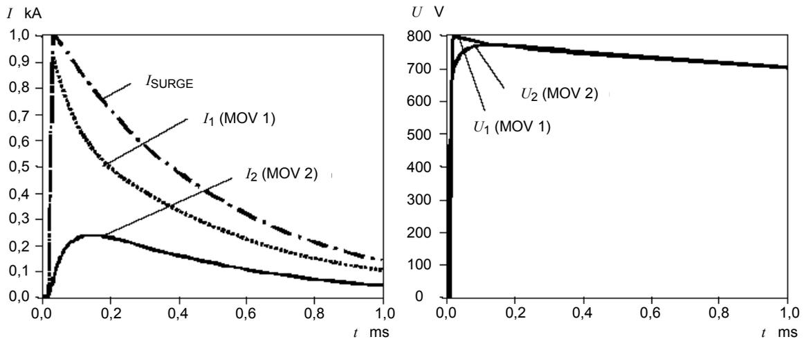
Figure C.4b – Current and voltage characteristics at MOV 1 and MOV 2 from 10/350  $\mu$ s surge
