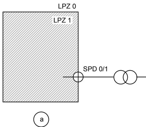
NOTE Figure 4a shows a structure powered by a transformer. If the transformer is placed outside the structure, only the low voltage lines entering the structure need protection by SPD. If the transformer should be placed inside the structure, the owner of the building often is not allowed to adopt protection measures on the high voltage side.
