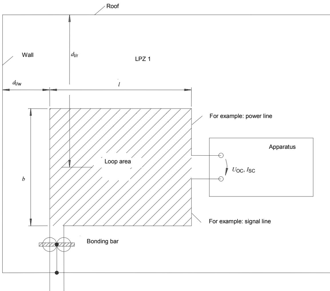
**Figure A.14 – Voltages and currents induced into a loop built by lines**
