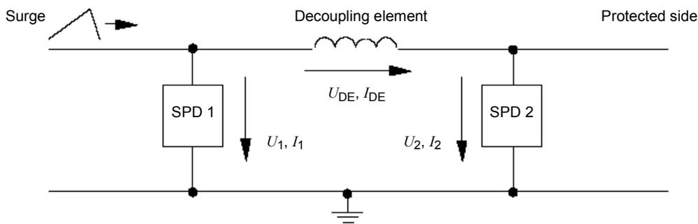
**Figure C.2 – Basic model for energy coordination of SPD**
