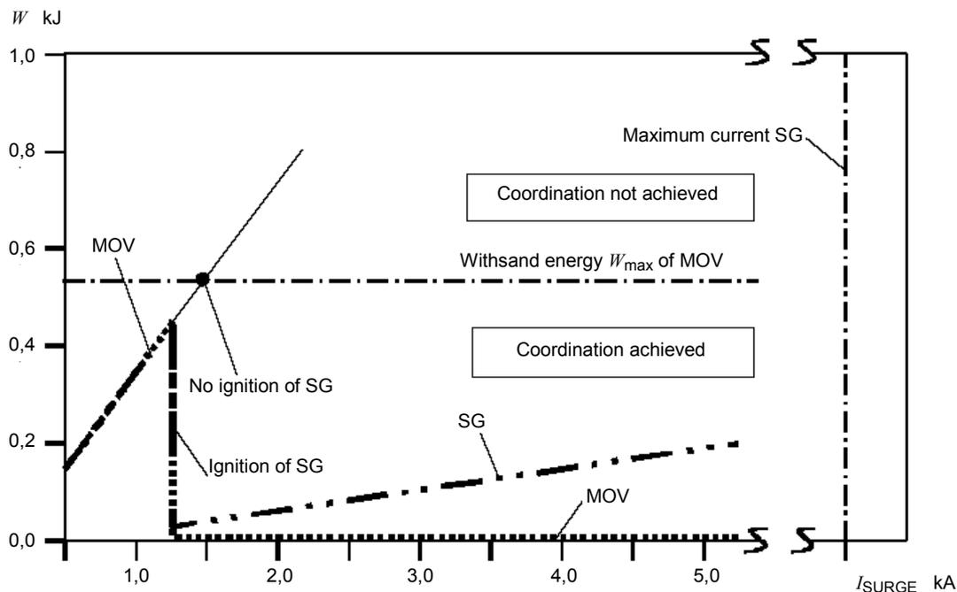
Figure C.5b – Principle for energy coordination of a spark gap and a MOV
