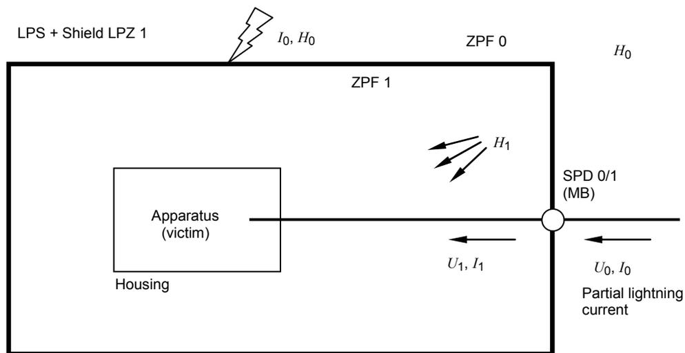
Figure 2b – LPMS using spatial shield of LPZ 1 and SPD protection at entry of LPZ 1 – Apparatus protected against conducted surges ( $U_1 < U_0$  and  $I_1 < I_0$ ) and against radiated magnetic fields ( $H_1 < H_0$ )
