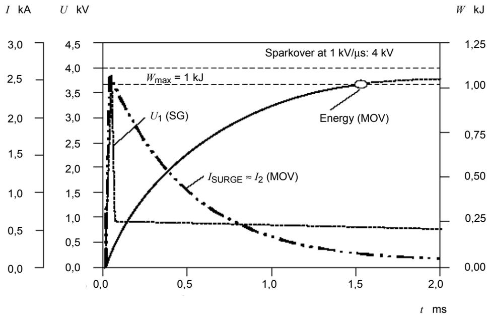
Figure C.8b – Current/voltage/energy characteristics for  $L_{DE} = 8 \mu H$  – Energy coordination for a 10/350 surge not achieved (spark gap not ignited)
